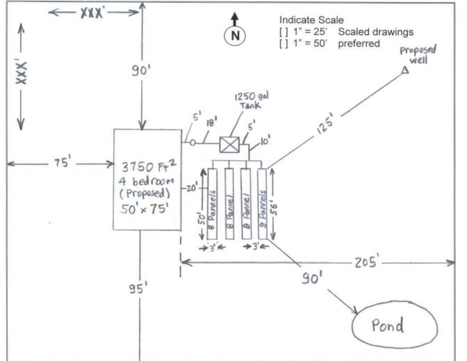
(Sewage flow) ÷ (absorption rate) ÷ (absorptive area) x (0.6 [leaching chamber efficiency]) = trench length
